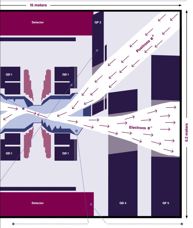
Bending the beams allows them to collide head-on, but it also creates synchrotron radiation that would cause background signals in the detector and confuse the analysis of the actual collision data. For this reason, the beam pipe has a series of ramps, or radiation masks, to shield the detector from the unwanted radiation.
